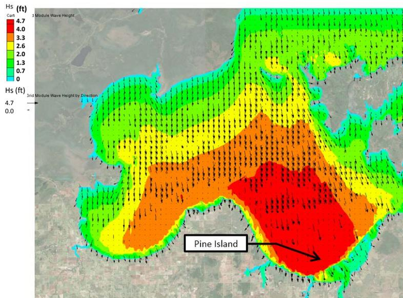
**Figure 13 – Modeled wave heights (Hs, in feet) for 19-Jun-2004**
