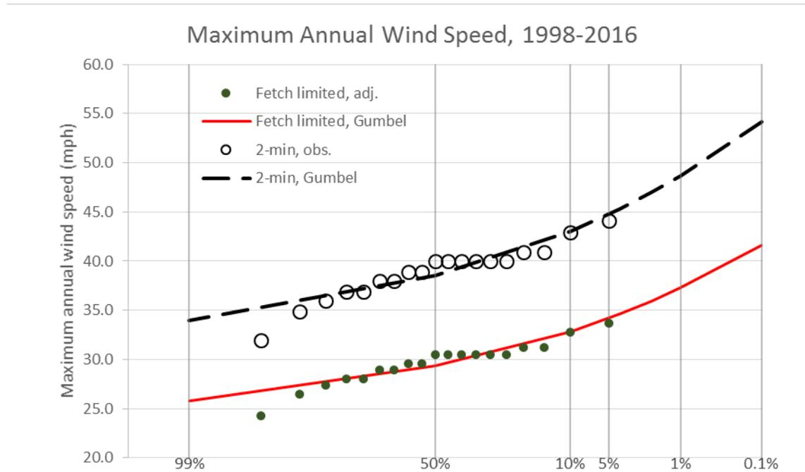
Figure 11 – Maximum annual 2-minute wind speeds and adjusted fetch-limited wind speeds fitted to Gumbel Distribution
