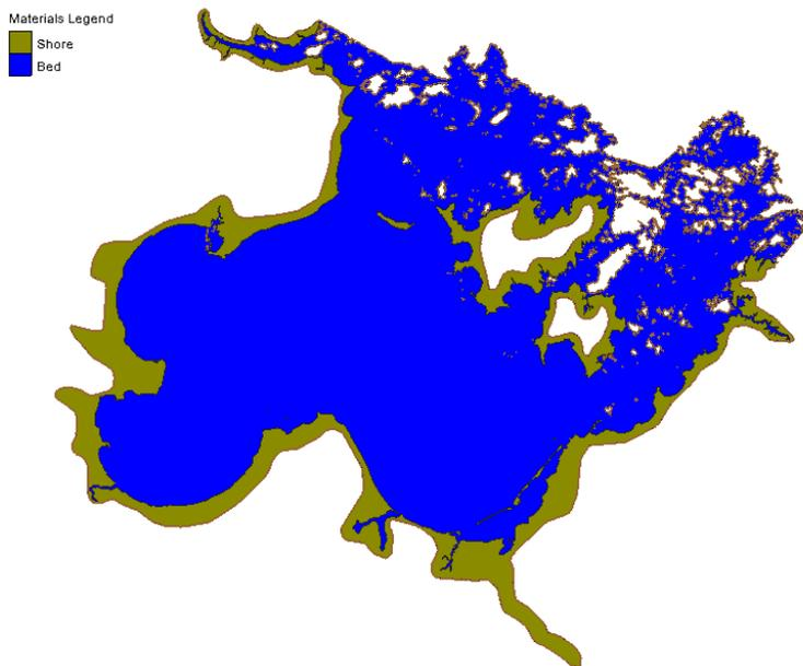
**Figure 5 – Material types for different roughness values in the AdH model**
