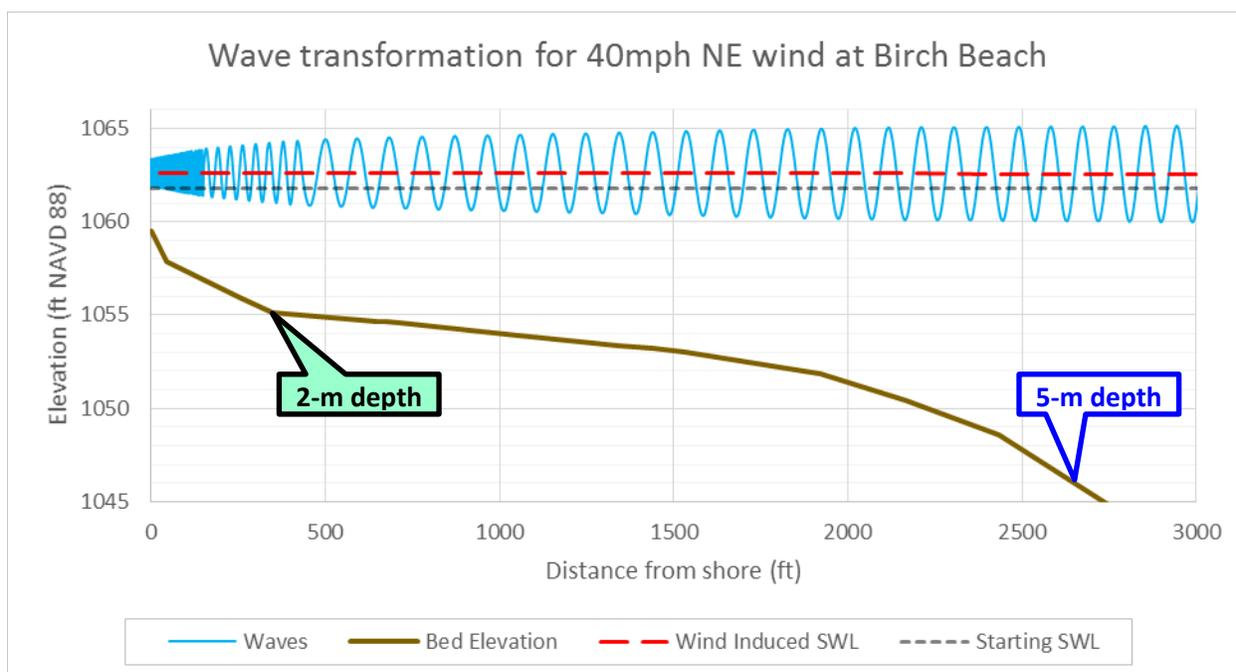
Figure 18 – Example of wave transformation as waves approach Birch Beach from wind from the NE at 40 mph
