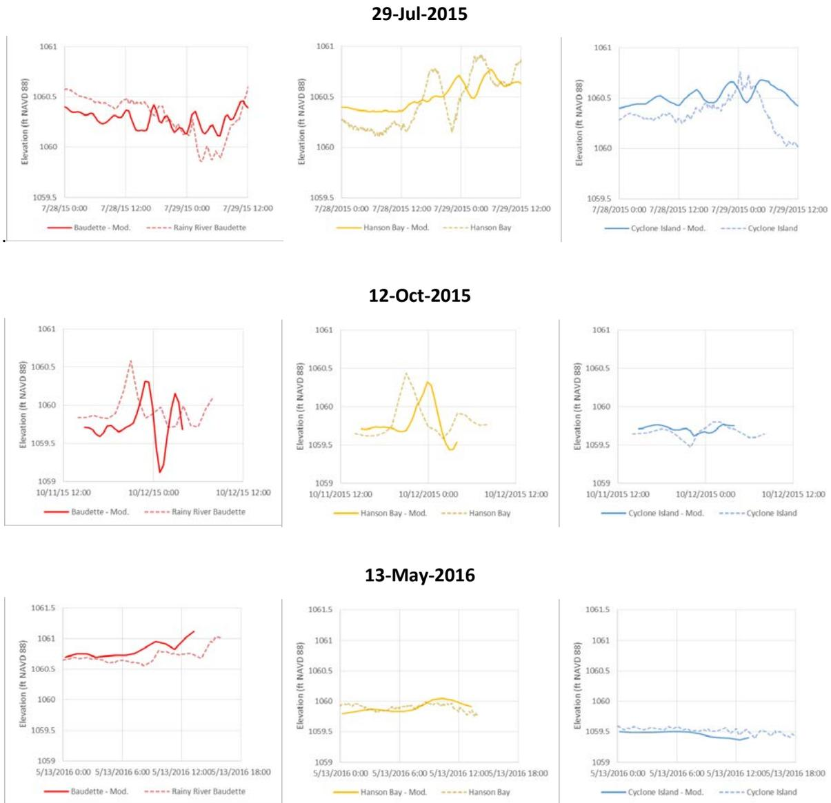
Figure 17 – Validation results for the wind setup model for three events in July 2015, October 2015, and May 2016
