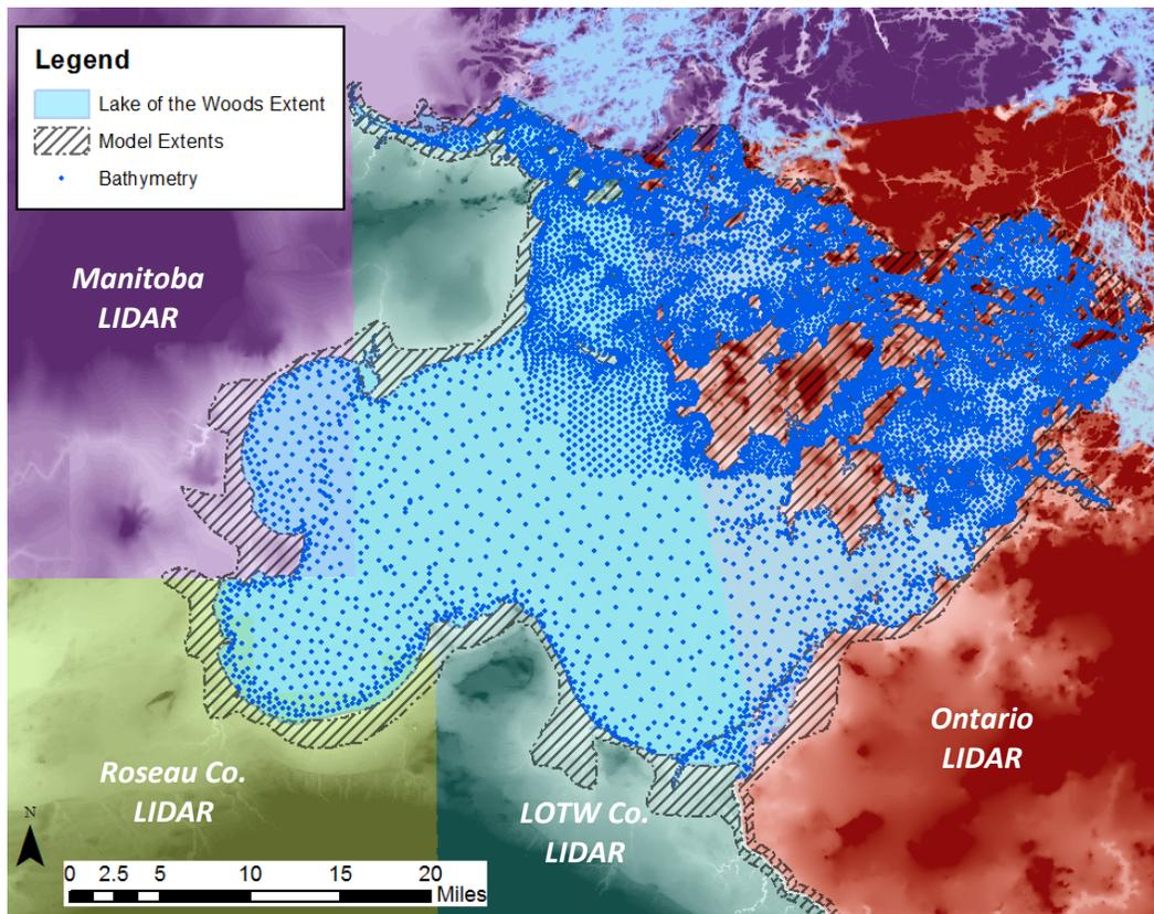
Figure 3 – Bathymetric and Ground Elevation Data Sources
