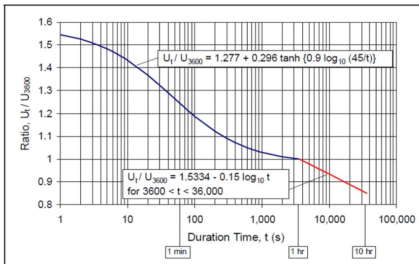
Figure 10 – Adjustment for wind speed data based on duration, from the Coastal Engineering Manual
